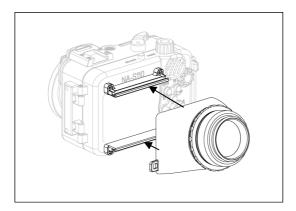
Attach the 25106 LCD Magnifier onto the rails above and below the LCD monitor window.
