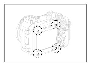
1. Remove the four rubber caps from the rear housing.
